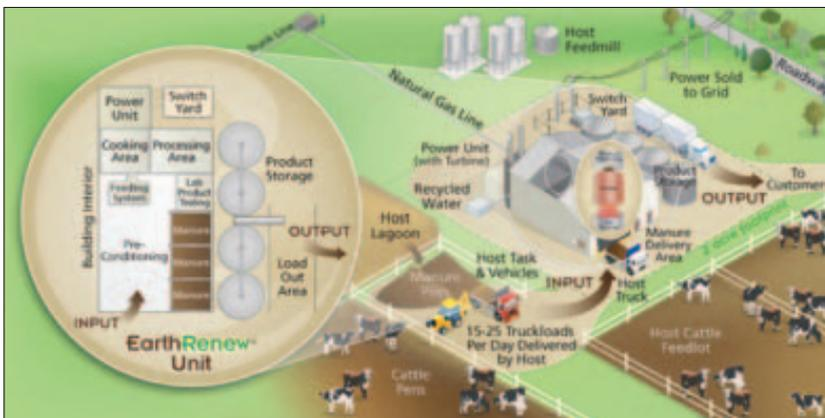
**GOOD COOK:** This diagram depicts installation of an EarthRenew unit at a typical dairy or feedlot. The system "cooks" manure into a pelleted fertilizer and produces electricity in the process, which can be sold to offset fuel costs.
